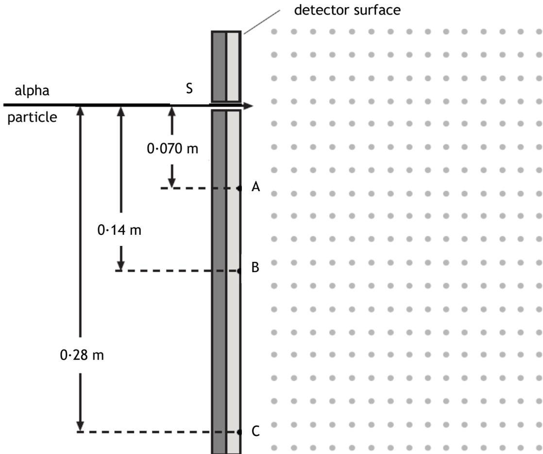
This magnetic field causes the alpha particle to travel in a semi-circular path and hit the detector surface.
