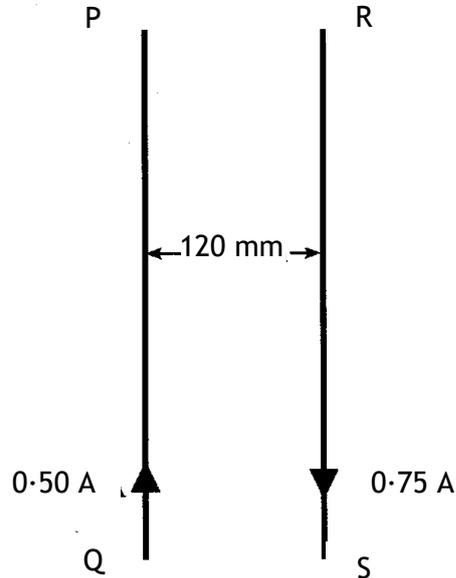
Conductor RS carries a current of 0.75 A in the opposite direction to the current in PQ.
