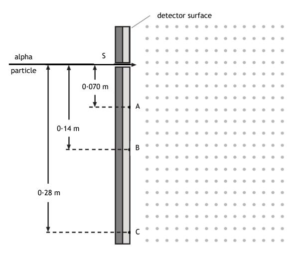
This magnetic field causes the alpha particle to travel in a semi-circular path and hit the detector surface.
