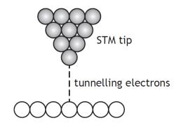
According to classical physics, electrons should not be able to cross the gap as the kinetic energy of each electron is insufficient to overcome the repulsion between electrons in the STM tip and the surface.
