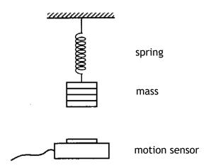
The mass moves with simple harmonic motion. The displacement-time graph of the mass is shown below.
