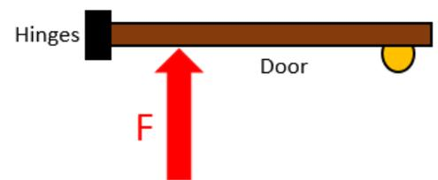
The door on the left will open more quickly than the door on the right because the force has been applied at a larger radius to the axis of rotation.
