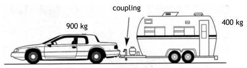
Calculate the tension in the coupling.
