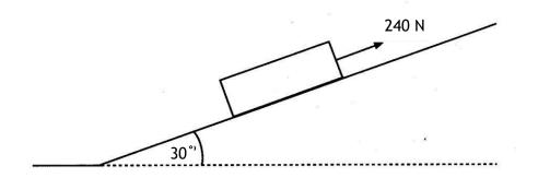
A force of 240 N is applied to the crate parallel to the slope. The crate moves at a constant speed of  $3 \cdot 0 \text{ ms}^{-1}$ .
