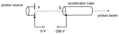
Protons released from the proton source start from rest at P.A potential difference of 200 kV is maintained between P and Q.
