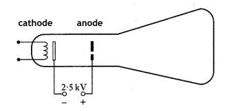
Assuming that the electrons start from rest at the cathode, calculate the speed of an electron just as it reaches the anode.
