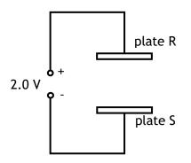
An electron is moved from plate R to plate S. Calculate the gain in kinetic energy of the electron.
