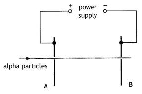
An alpha particle travelling at a speed of  $2.60 \times 10^6$  ms<sup>-1</sup> passes through a hole in plate A. The mass of an alpha particle is  $6.64 \times 10^{-27}$  kg and its charge is  $3.20 \times 10^{-19}$  C.
