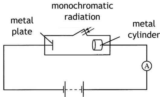
There is a constant potential difference between the metal plate and the metal cylinder. Photoelectrons produced at the plate are collected by the cylinder. The frequency of the radiation is set at a value above the threshold frequency.
