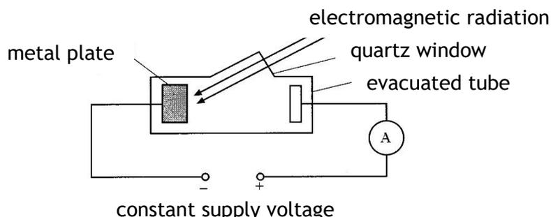
When light of wavelength 605 nm is incident on the metal plate, electrons are released with zero kinetic energy.
