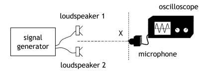
The microphone is initially placed at point X, which is the same distance from each loudspeaker. A maximum is detected at X.
