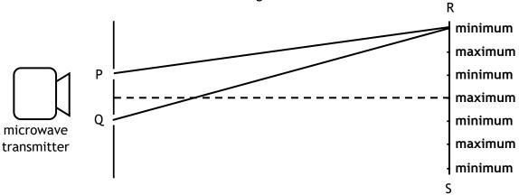
A microwave receiver is moved between R and S and a series of maxima and minima are detected, as shown.
