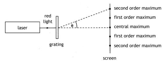
A series of maxima and minima are observed. Explain in terms of waves how a minimum is produced.
