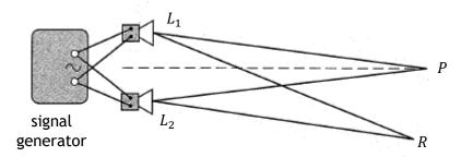
At position P, which is the same distance from both loudspeakers, the microphone measures a maximum intensity of sound. The next maximum is registered at position R, where  $L_1R=4\cdot 6\ m$  and  $L_2R=4\cdot 3\ m$ .
