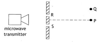
The microwave detector is moved and the **next** maximum is recorded at Q. The path difference (SQ - RQ) must be
