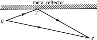
An interference pattern is produced.
