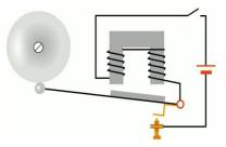
When the school bell rings it depends on an electromagnet. When the circuit is closed the magnet created attracts the piece of steel on the hammer, which strikes the bell when it moves up. As it moves up the circuit is broken so that the magnet no longer works.
