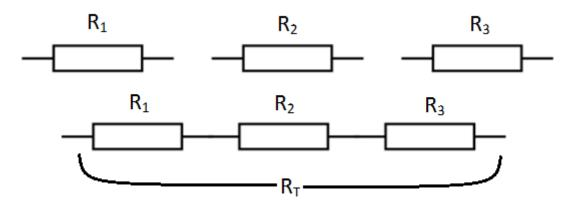
If we join components in series we increase the resistance of the circuit.
