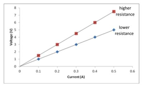
The relationship between the resistance of a conductor, the voltage across it and the current through it is:
