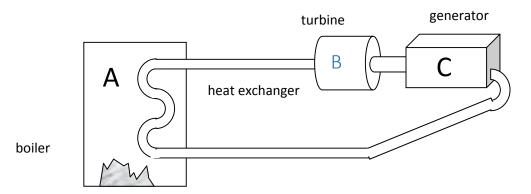
In a thermal power station we burn fuel to produce heat.
