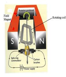
A motor depends on the interaction between two magnetic fields. The coil in the centre of the motor is an electromagnet. When current flows through the rotating coil its magnetic field interacts with the field from the field magnet (which can be permanent or an electromagnet).
