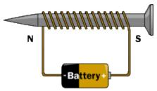
Permanent magnets cannot be turned off. An electromagnet can be switched on and off. A length of wire is wrapped around a piece of iron, for example a nail. The current which flows through the wire causes a magnetic field around the nail which is similar to that of a bar magnet.
