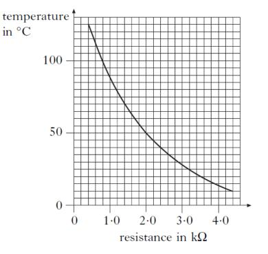
The thermistor is connected in a circuit. At a temperature of 50  $^{\circ}$ C, the current in the thermistor is 4 mA.
