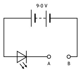
In normal operation, the LED carries a current of 20 mA and the voltage across it is 1.9 V.
