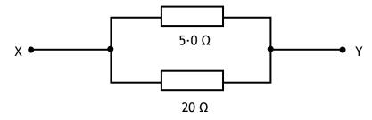
Calculate the total resistance between X and Y.
