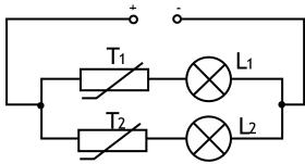
The resistance of a thermistor decreases when the temperature increases.
