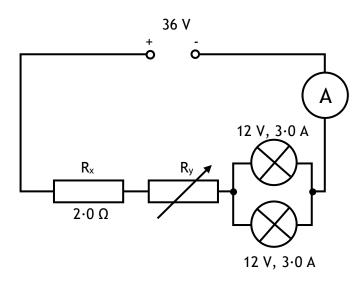
Explain why the resistance of R<sub>y</sub> has to be adjusted to allow both lamps to operate correctly.
