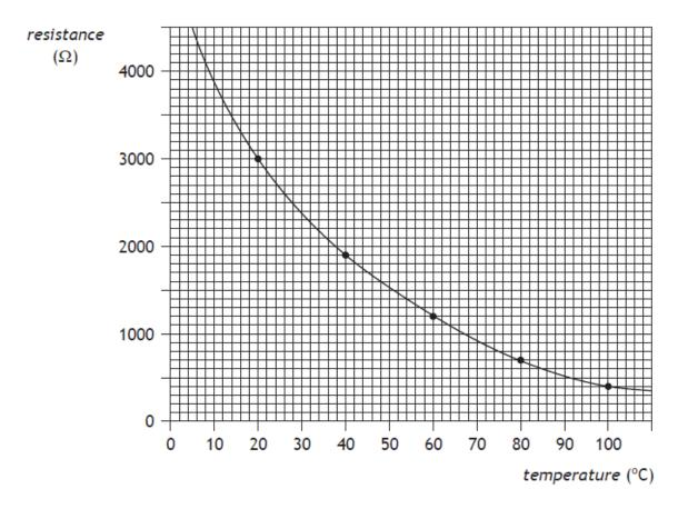
Use the graph to determine the temperature of the water when the voltage across the thermistor is 2.0 V.
